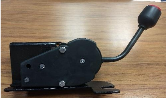
Current shifter setup rotated to drill new 11/32" hole
