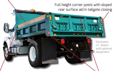
Board pocket design aligns with cabshield and allows the use of tapered side boards to increase capacity when hauling lighter loads such as brush, firewood, and mulch
