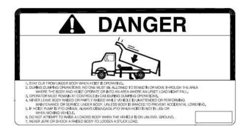
**WARNING:** Missing or damaged decals can lead to accidents which may cause serious injury or death. If any decals are missing or damaged, they must be replaced.
